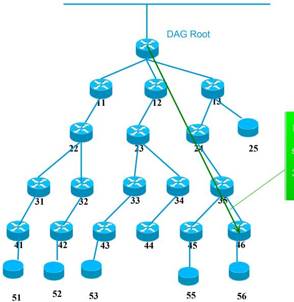
New (projected) DAO with path segment unicast to target 56 via 35 (ingress) and 46 (egress)
