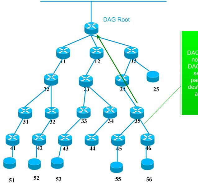
DAO-ACK (alt: non storing DAO) unicast, self 35 as parent, final destination 56 as target Applicatio
