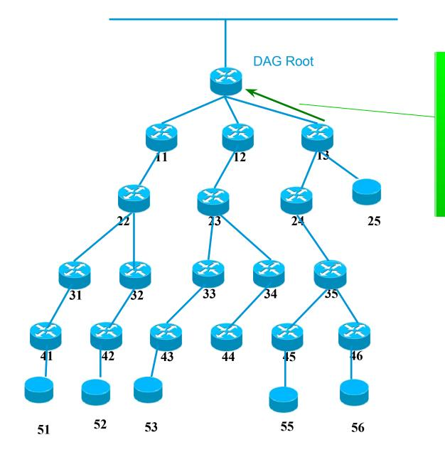
DAO-ACK (alt: non storing DAO) unicast, self 13 as parent, final destination 56 as target
