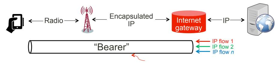
A bearer encapsulates a user's IP flows. A 'default bearer' is set up for every handset.
