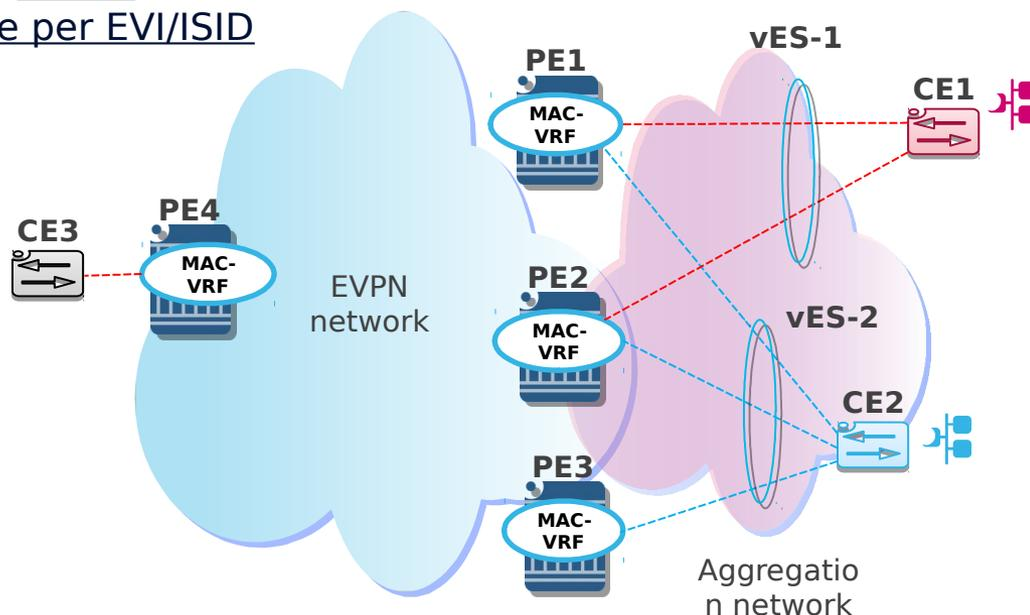
The user must be able to configure a given ES with a “revertive” or “non-revertive” operation. Non-revertive avoids service impact when an ES comes back up.
