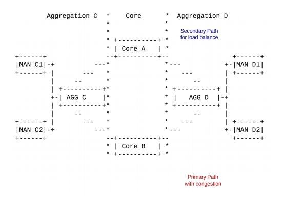
Load balancing between Aggregation and Core
