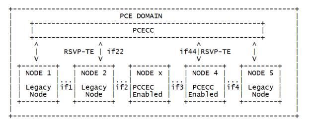
o Node1 sends a path request message for the setup of LSP which has destination as Node5.
