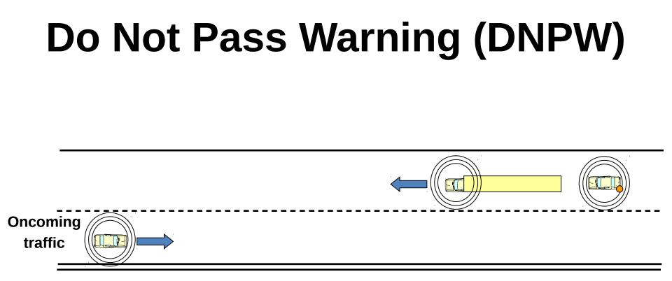
When showing intent to move to oncoming lane, driver receives warning if not safe to pass.
