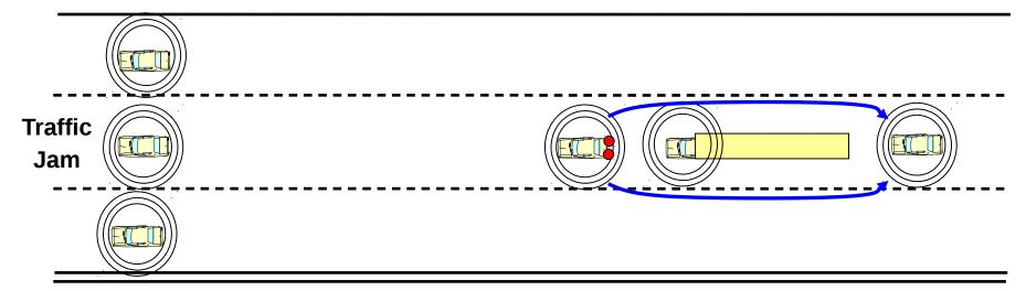
High deceleration by car approaching jam. Trailing car Informed via DSRC within 100 msec.
