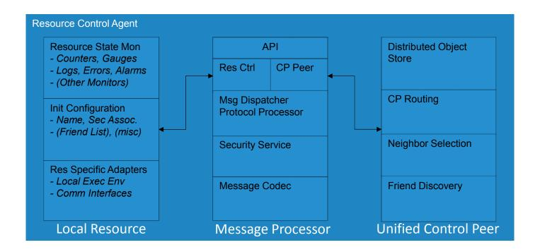
Two faces of the RCA: the RCA acts both as an interface to the local resource that it controls, and as a building block of the control plane spanning all resources within the control domain (unified control peer).
