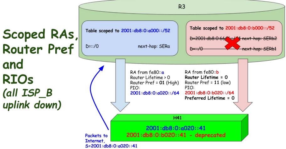
**R**3 Scoped RAs, Table scoped to 2001:db8:0:b000::/52 Table scoped to 2001:db8:0:a000::/52 D=2001:db8:0:66 **Router Pref** D=::/0 ext-hop: SERa D=::/0 ext-hop: SERb1 and **RIOs** RA from fe80::b RA from fe80::a Router Lifetime = 0 Router Lifetime = 0 PIO: PIO: (all uplinks 2001:db8:0:a020::/64 2001:db8:0:b020::/64 Preferred Lifetime = 0 Preferred Lifetime = 0 down) H41 2001:db8:0:a020::41 - deprecated 2001:db8:0:b020::41 - deprecated Broken intra-site communication!
