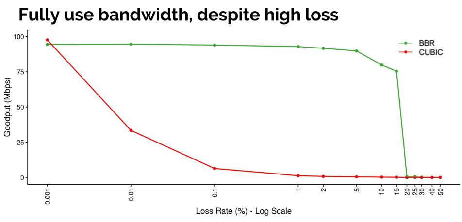
BBR vs CUBIC: synthetic bulk TCP test with 1 flow, bottleneck\_bw 100Mbps, RTT 100ms
