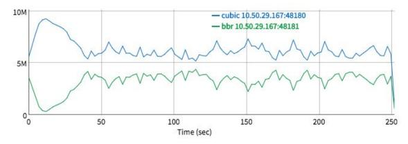
At first CUBIC/Reno gains an advantage by filling deep buffers
