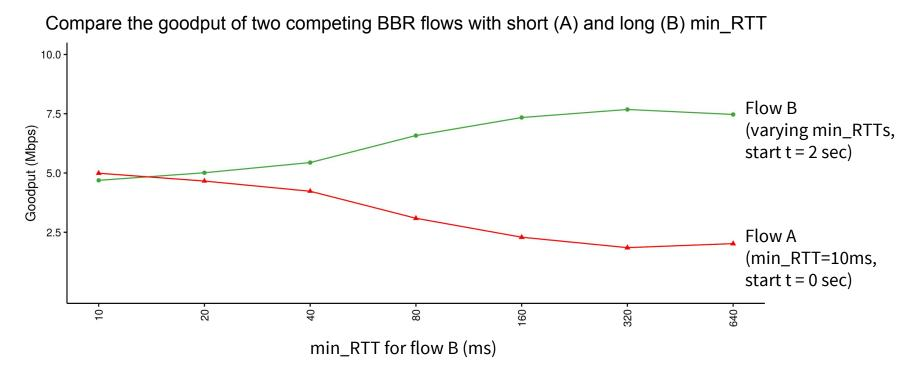
BBR flows w/ higher RTT have an advantage; but BBR flow with 64x higher min\_RTT only has <4x higher bw bw = 10 Mbit/sec, buffer = 1000 packets
