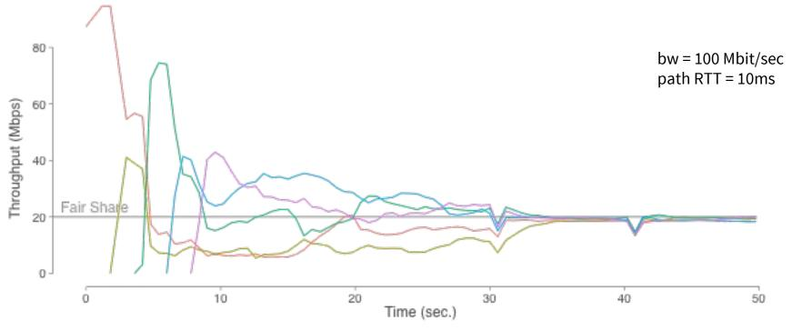
Converge by sync'd PROBE\_RTT + randomized cycling phases in PROBE\_BW
