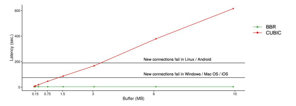
BBR vs CUBIC: synthetic bulk TCP test with 8 flows, bottleneck\_bw=128kbps, RTT=40ms
