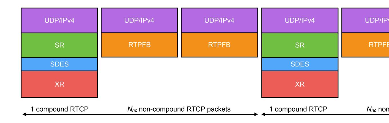
• Average RTCP packet size,  $S_{rtcp} = (S_c + N_{nc} \times S_{nc}) / (1 + N_{nc})$ where  $N_{nc} = 0$  if non-compound packets are not sent
