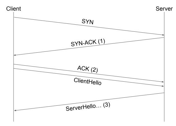
In TLS over TCP, client proves ownership of IP address before sending ServerHello...Finished flight:
