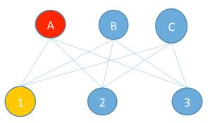
Consider tree 2, and say node A is the tree root. Now, consider what happens if Node 1 goes down? During tree calculation, because the prior tree calculation used Node 2 as the parent, the policy selection step continues to select Node 2 as the parent in new tree calculations.
