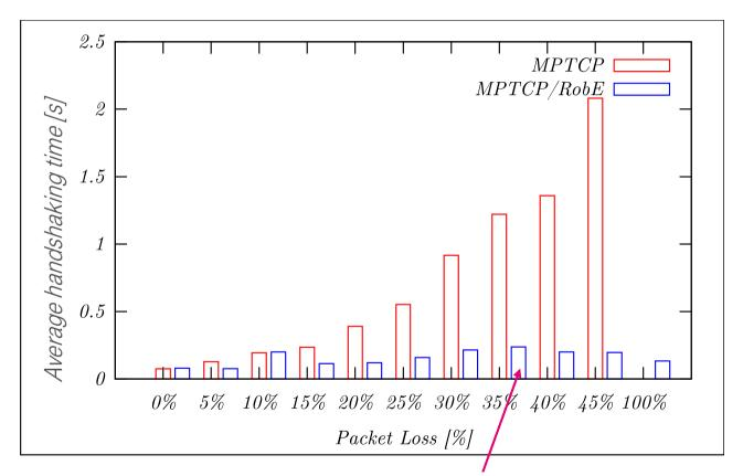
RobE should stay stable over time, here it is not fully the case because impl. and setup is still imperfect.
