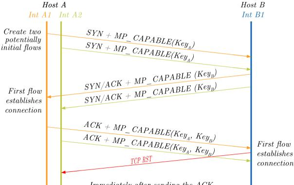
Immediately after sending the ACK, subflows are established on every path as defined in RFC 6824.
