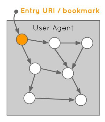
Application as finite-state machine (FSM) at the client
