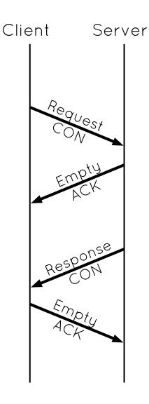
ACKs are **empty** when the code is zero 0.00 0x4712 2.05 0x0815 Token: 0xBEEF00 Content-Format: text/plain hello separate 0xFF
