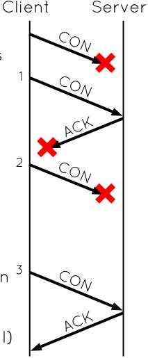
Receiver must send an Acknowledgement (ACK) for CONs
