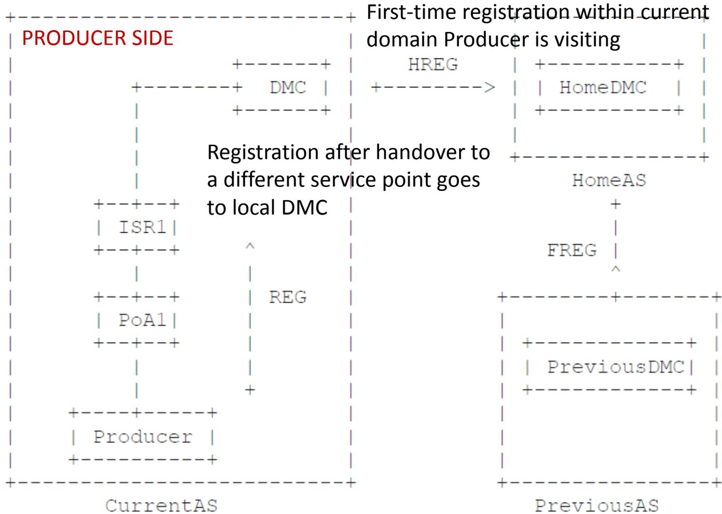
Inter-domain handover triggers timeout-based flushing of registration entries associated with Producer, and re-direct to new domain
