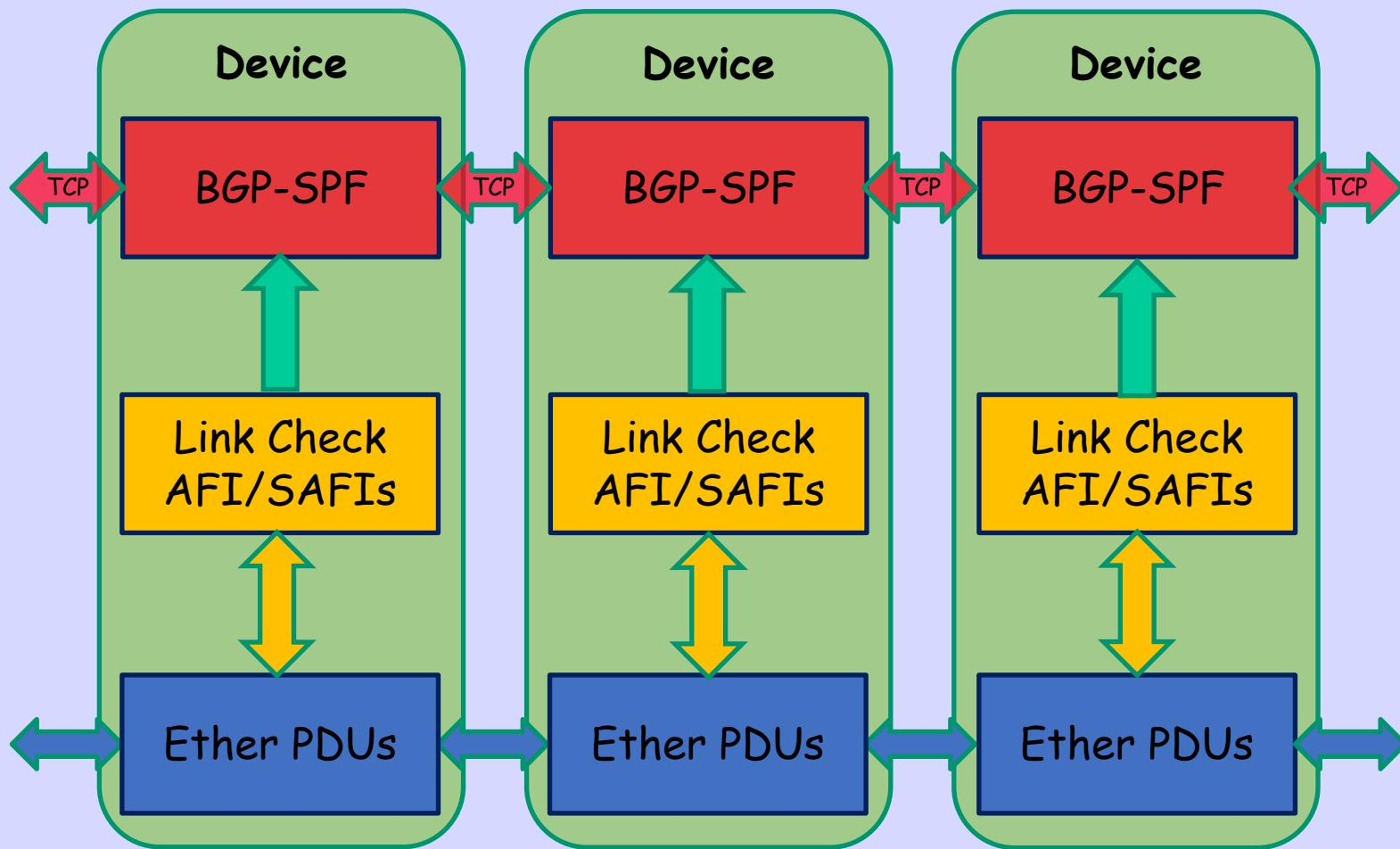
MAC Link State exchanged over raw Ethernet and pushed up stack
