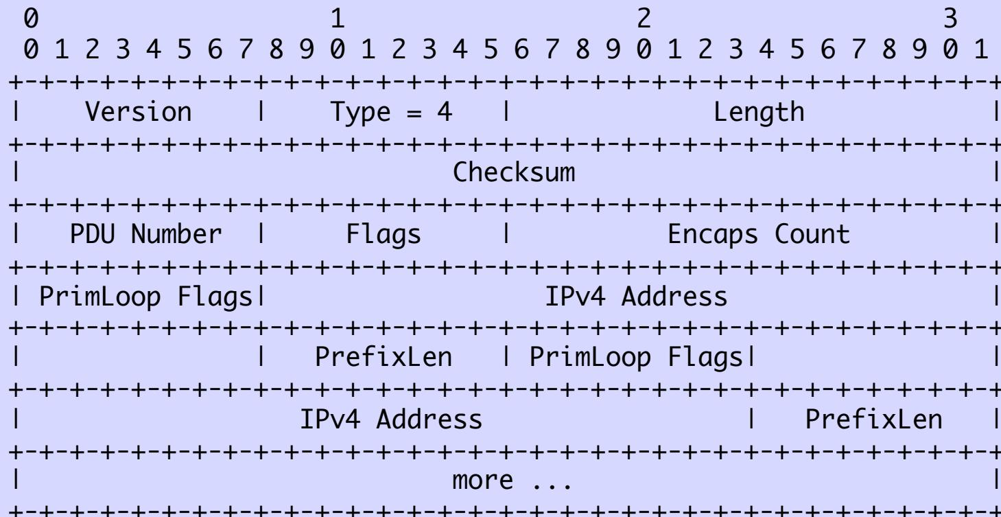
An Encapsulation message describes zero or more addresses of the encapsulation type.
