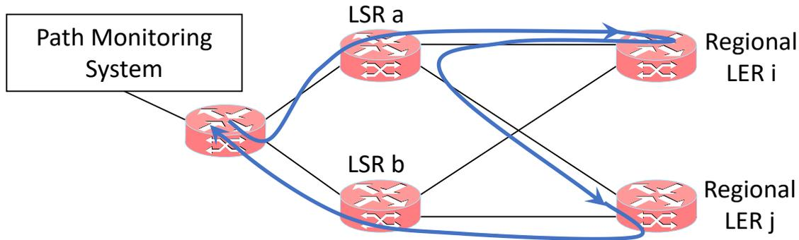
Detection of events (different measurement paths combine as shown below to create an individual measurement path combination per monitored interface):
