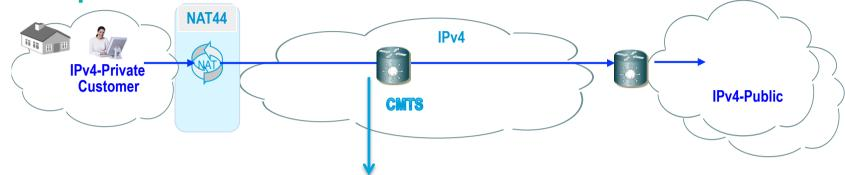
Inbound Security IP ACL applied to cable bundle interface for all subscribers
