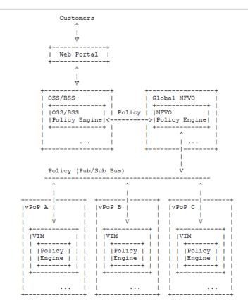
Figure 6: Simplified view of a service provider's NFV Architecture:
