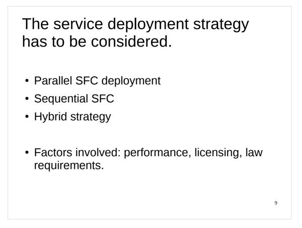
One possible approach is to deploy all the VNFs of a given service function chain in a single server and deploy as many of these servers in parallel in order to server the different flows.
